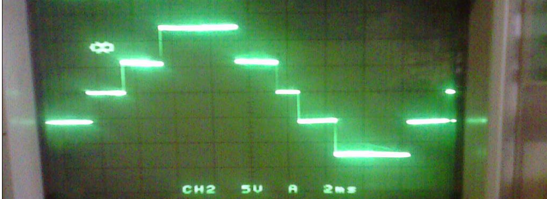
Figure 16: Experimented waveforms of 5-level line-to-line Output voltage of the MLI
