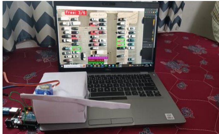
Figure 24: Gate Control Servo at “CLOSED” state
