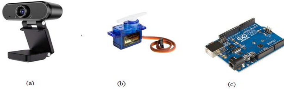
Figure 3: (a) Webcam (b) Servo Motor (c) Arduino (source: Google Images)
