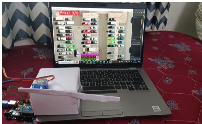
Figure 6: Hardware Implementation of Parking Management System
