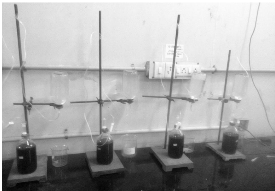
Figure 1: Experimental Setup for Biogas Production
