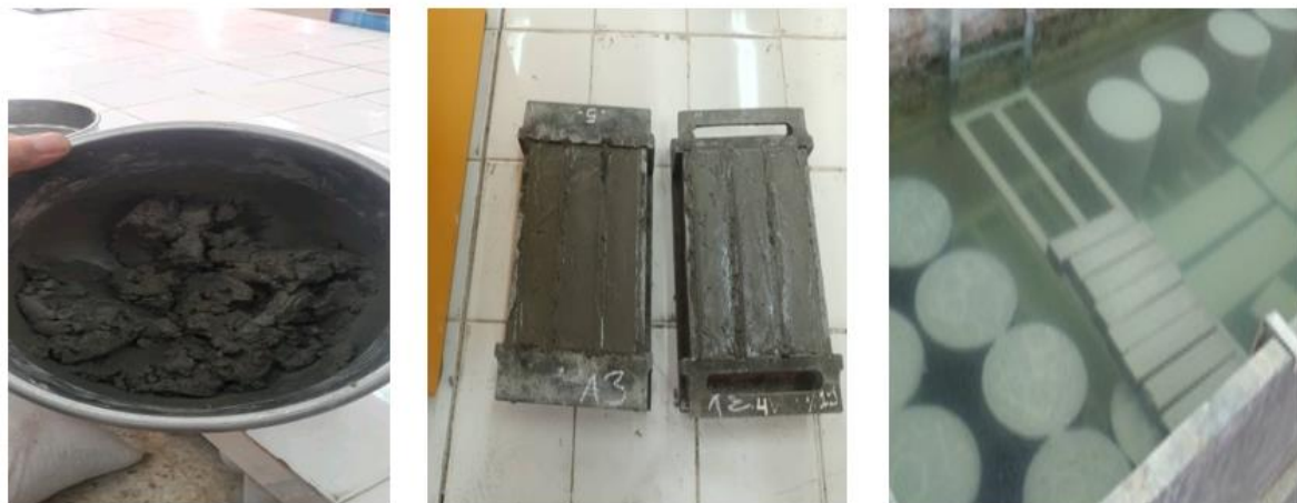
Fig 4: Mixing of mortar, filling of molds and conservation of mortar specimens
