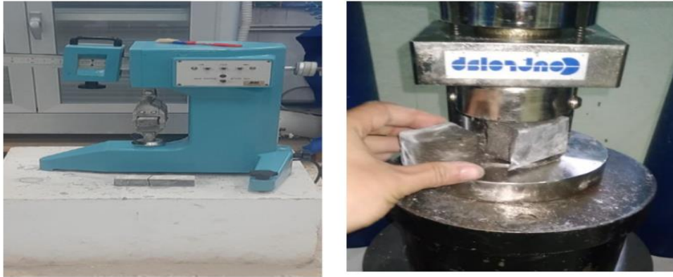
Fig 5: Bending and compression tests.
