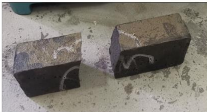
Fig 6: Failure of an ordinary mortar subjected to tension by bending.
