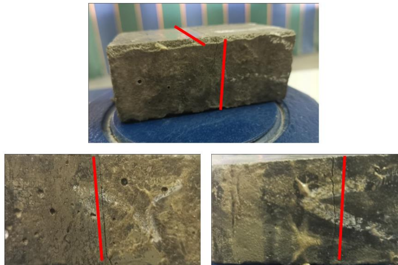
Fig 7: Failure of a mortar reinforced with steel fibers subjected to tension by bending
