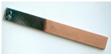
Fig 2: Copper deposit on XC18 flat specimen.
