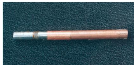
Fig 3: Copper deposit on E34 cylindrical specimen.
