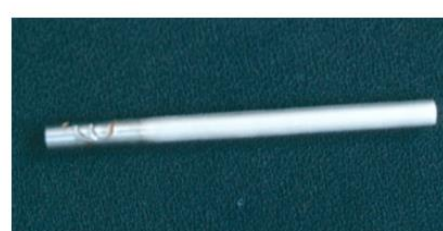
Fig 5: Nickel deposit on E34 cylindrical specimen.
